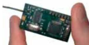
KNX RF circuit / KNX RF circuit
